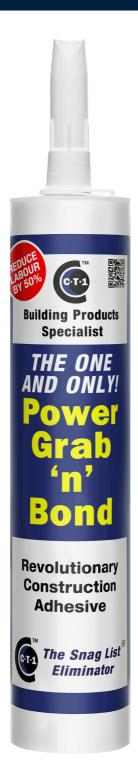
Density: 1569kg/m3 Curing in 24hrs: 2 to 3mm Shrinkage: None **Skinning Time:** 10-15mins E-Modulus 100%: 1.39 Mpa Volume shrinkage after cure: none Hardness - DIN 53505 Shore A: 60° Tensile strength: 22Kg / cm<sup>2</sup> Thermal stability: -40°C till + 90°C
